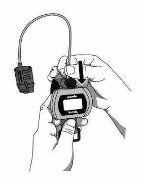
Turning on the oximeter with the finger in the probe
