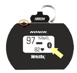
**Note:** Be sure you hold down the button for at least 3 seconds. By doing this the oximeter will avoid a state where the oximeter won't allow a Bluetooth connection to occur. Oximeter units with serial numbers 501924607 and larger do not run the risk of entering this state.
